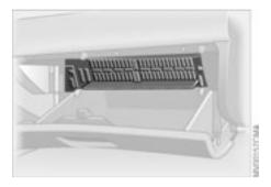
You will find the fuses and information on their respective allocation in the glove compartment behind a panel with two snap clips.
